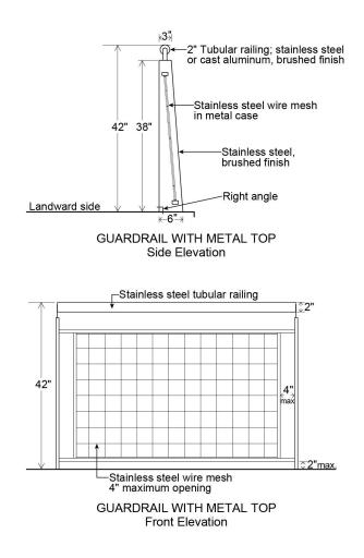
All guardrail components and hardware shall be in No. 316 Stainless Steel, passivated and bead blasted.
