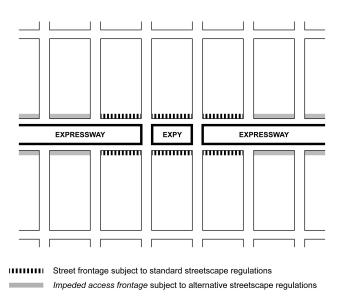
DIAGRAM ILLUSTRATING IMPEDED ACCESS FRONTAGE
