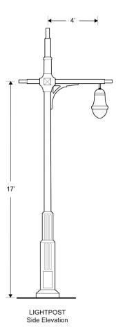
The lightpost shall conform to the street lighting standard drawings for a 17 foot "TBTA" short pole with "Tear Drop Luminare" set forth by the DOT.
