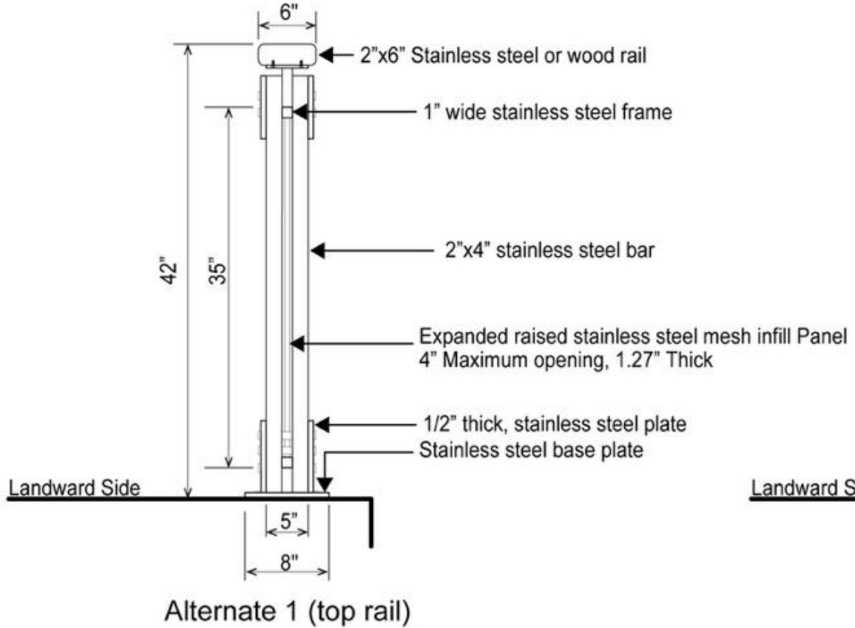
All guardrail components and hardware shall be in unpainted stainless steel and shall conform to any additional standards set forth by DPR.
