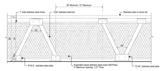
GUARDRAIL (TYPICAL) Front Elevation
