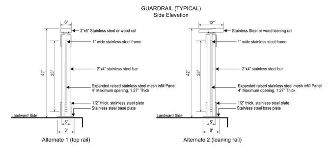
All guardrail components and hardware shall be in unpainted stainless steel and shall conform to any additional standards set forth by DPR.
