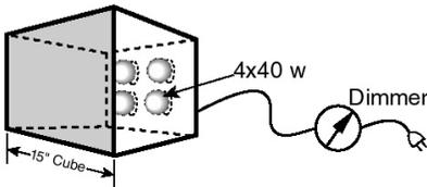
To calibrate, build a lightbox as shown above. The front of the box shall be 1/4" #2447 opal plexiglass; the other five interior sides shall be painted matte white.
