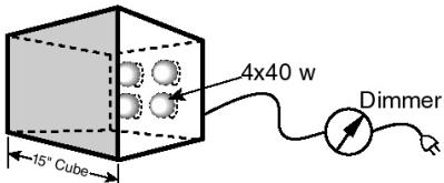
To calibrate, build a lightbox as shown above. The front of the box shall be 1/4" #2447 opal plexiglass; the other five interior sides shall be painted matte white.
