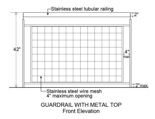
All guardrail components and hardware shall be in No. 316 Stainless Steel, passivated and bead blasted.
