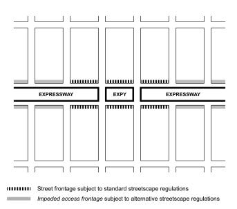
DIAGRAM ILLUSTRATING IMPEDED ACCESS FRONTAGE
