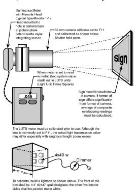
Four standard 40 watt 120 volt incandescent lamps shall be mounted on the back of the box and wired through a dimmer
